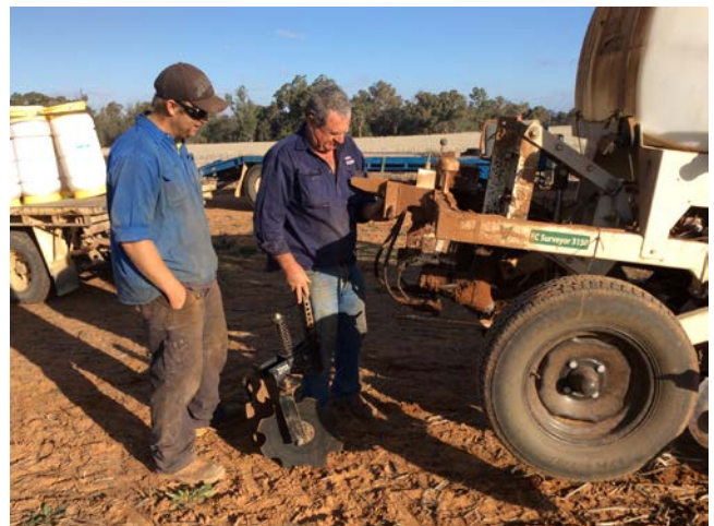
Grower, Rod Morton, is shown how the Veris unit maps pH and electrical conductivity prior to surveying his 120 ha paddock going into canola in 2016.
