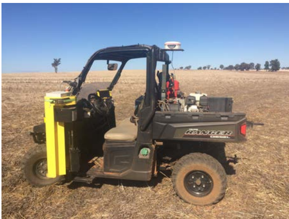
Precision Agriculture survey McKinley's 260 Ha barley paddock in May 2016 on a 2 Ha grid for pH and Phosphorus
